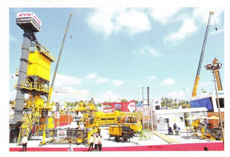
ew product on display was the compact batching plant with sidewall conveyors, which can achieve a steep angle up to 50 degrees as compared to the 17-18 degree by conventional conveyors. It gives a 10% better output as compared to other batching plants. With this new sidewall conveyor, the batching time is reduced to 50 seconds since the conveyor is very short and runs at a very high speed. The plant gives higher productivity, lower fuel consumption, and enables easy application in constrained
