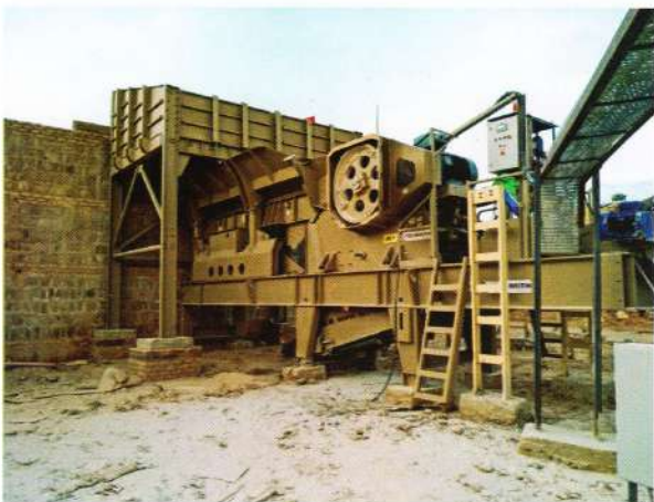
▲ TIL H3244 PP is a wheel mounted electric powered primary crushing & screening unit.
