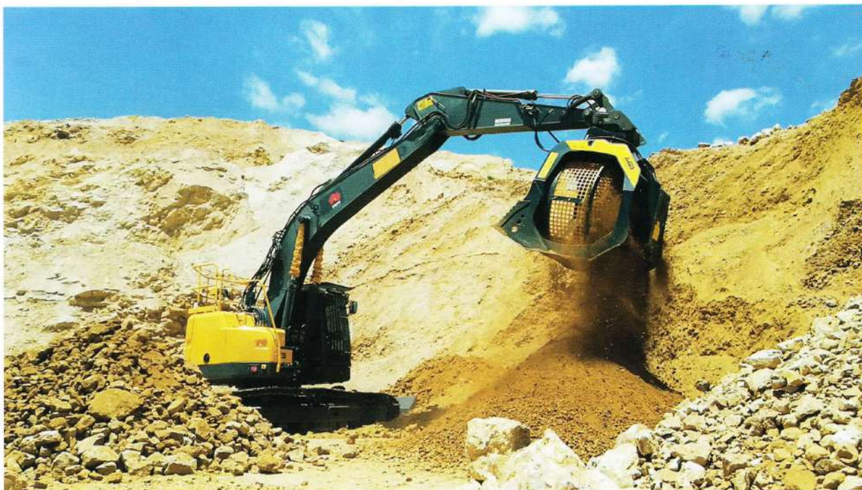
▲ The MB-S18 screening bucket has been designed for medium and large-scale contexts that require high performance and large-scale production.
