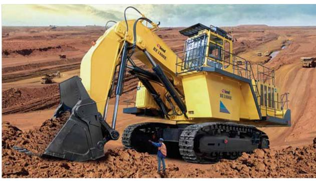
▲ BEML180 ton Electric Hydraulic Excavator BE 1800E is the largest excavator available.
