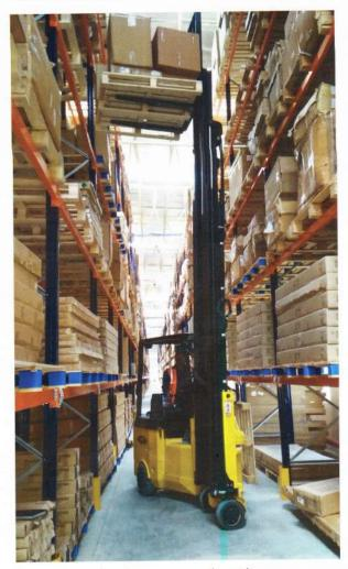
Articulated Truck working in narrow working aisles
