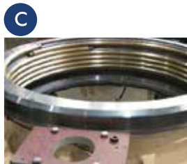
PATENTED FIELD REPLACEABLE BRASS THREADS Older machines use steel-on-steel rotation threads that frequently gall or weld together. KPI-JCI's patented a brass-thread insert resists the galling and welding.
