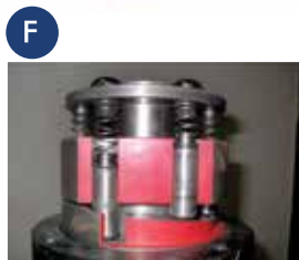
ANTI-SPIN CONE BRAKE Anti-spin feature reduces manganese wear cost and minimizes projectiles for improved safety. Optional hydraulic anti-spin also available
