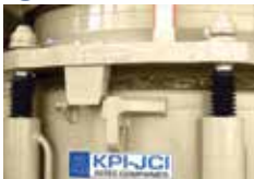
TRAMP IRON RELIEF SYSTEM Eliminates maintenance costs associated with accumulators. Pressure relief valves act as a latch, generating minimal back pressure build-up during an overload event. Picture above shown in the "clearing" position.
