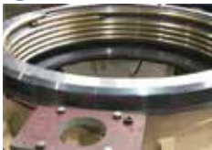
PATENTED FIELD REPLACEABLE BRASS THREADS Older machines use steel-on-steel rotation threads that frequently gall or weld together. KPI-JCI's patented brass-thread insert resists the galling and welding.
