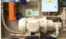
LUBE PANEL Houses lube pump, filter, etc. are away from the crusher in an easy to service panel.
