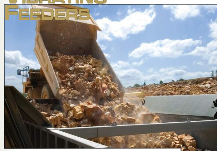
T elsmith feeders are available in sizes ranging from 36" x 12' up to 72" x 34', in a variety of models and configurations.
