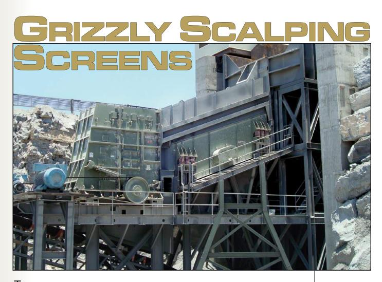
elsmith inclined grizzly scalping screens are most commonly utilized in conjunction with an apron or pan feeder, ahead of the primary crusher. Typically chosen when excessive clay or an abundance of fines are present, grizzly scalpers are capable of efficient scalping in the most difficult applications.
