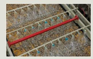
WASH SCREEN ARRANGEMENT: The typical arrangement would include spray pipes with nozzles and a water distribution manifold, mounted to the sub-frame, including shut-off valves and hoses.
