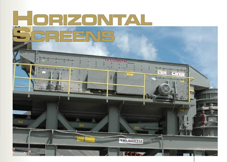
elsmith Horizontal Screens offer reliable, versatile performance in a variety of applications. The low horizontal profile is ideal for road portability on rubber tired portable or track mounted plants. Additionally, horizontal screens are often applied in critical sizing areas of stationary plants, or, where the ability to operate at high G-forces helps minimize blinding or assist in dewatering.
