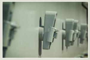
QuickLok<sup>®</sup> tensioning wedges are ideal for side tension media of all kinds. The double wedge design holds firmly during operation and allows quick media changes.
