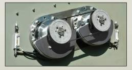
Oil level sight gauges are located outside of the guard protected area. Built into the sight gauge are oil drain, oil fill and grease zerk fittings for quick maintenance, including oil changes, without removing the guard.
